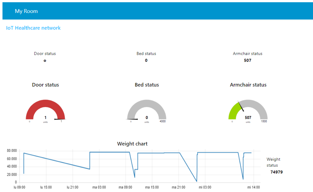
Figure 27. Dashboard of the Node-RED with the actual status of each sensor.
