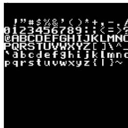
FIGURE 2. A .chr file containing a very simple tileset for the NES
