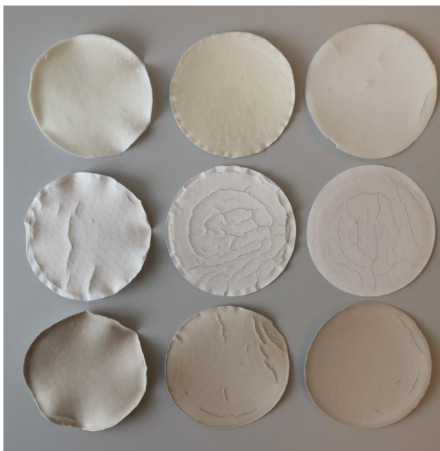
Figure 12. Cakes dried with different drying methods. An air-conditioned cake on the left, a grilled one in the middle and vacuum dried cake on the right. Bottom row MCC1, middle row MCC2 and top row MCC3.
