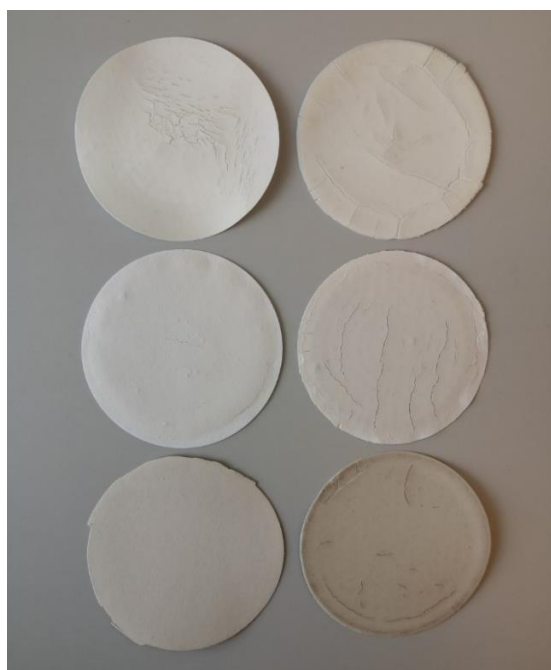
Figure 13. On the left side are rolled cakes and on the right side are compressed cakes. Both were dried in a vacuum dryer. Bottom row MCC1, middle row MCC2 and top row MCC3.
