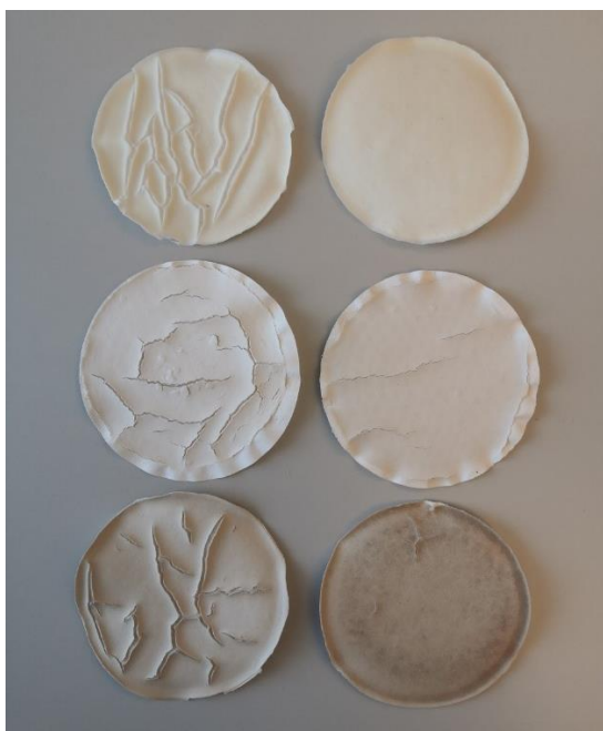
Figure 14. On the left side are rolled cakes and on the right side are compressed cakes. Both were dried in an air-conditioning room. Bottom row MCC1, middle row MCC2 and top row MCC3.
