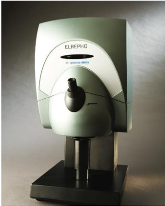
Figure 2. L&W Elrepho spectrophotometer. (ABB 2016)
