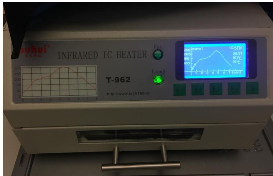
Figure 27: The board being heated inside a reflow heater for the solder paste to work
