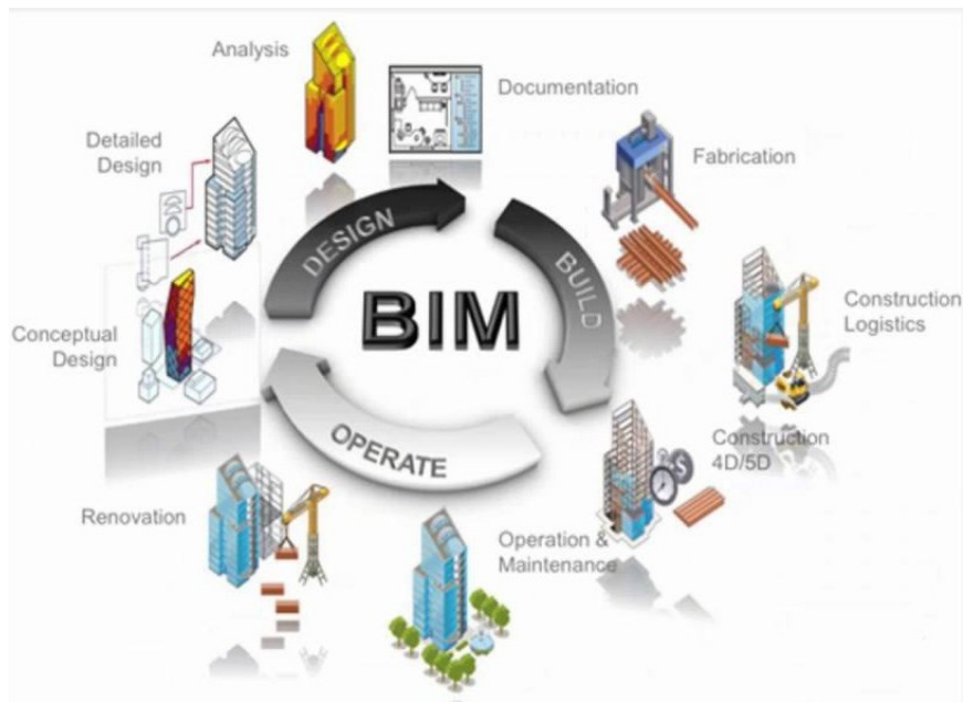
Figure 1. BIM cycle (Structural details, n.d.)
