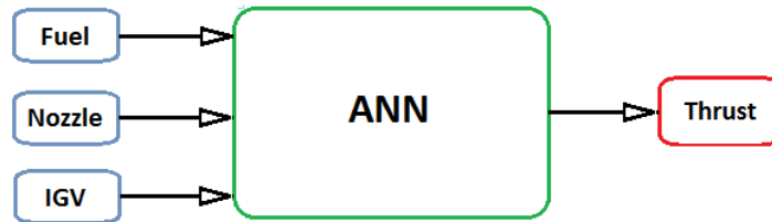
Figure 5. Block Diagram of an ANN -Based Model of an ADGT [48].
