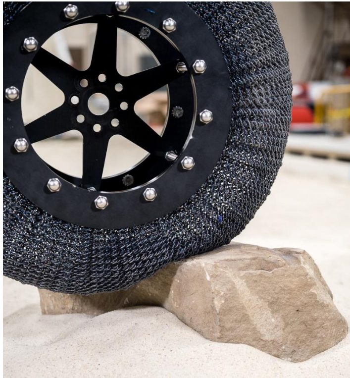
Figure 24. Picture of a Shape Memory Alloy wheel tire developed by NASA. (Credit: NASA)
