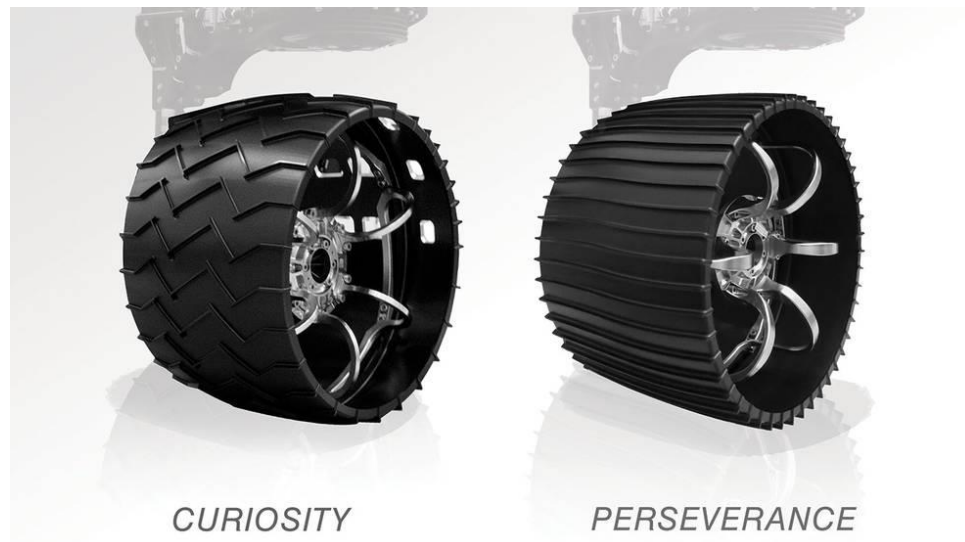
Figure 19. The aluminum wheels of NASA's Curiosity (left) and Perseverance rovers. (Credit: NASA/JPL-Caltech)
