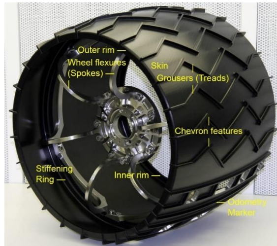
Figure 17. Diagram of the Curiosity's wheel. (Credit: NASA/JPL-Caltech/Emily Lakdawalla)
