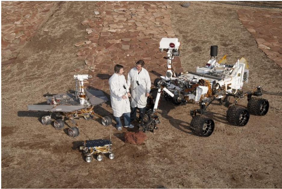
Figure 15. A picture of the three JPL Mars Rovers. Front and center is the flight spare of the Sojourner, Marie Curie. On the left is the Surface System Test Bed (SSTB) of the Mars Exploration Rover. At right is the Vehicle System Test Bed (VSTB) nearly identical to the Curiosity Rover [5]. (Credit: NASA/JPL-Caltech PIA15279)
