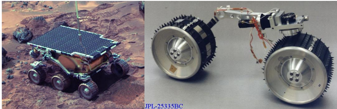
Figure 12. Picture of the Sojourner Rover near "The dice" (left). Picture of the Sojourner Rover Wheels (right). (Credit: NASA/JPL)
