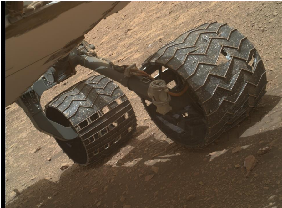
Figure 18. Curiosity's wheels punctures. (Credit: NASA)
