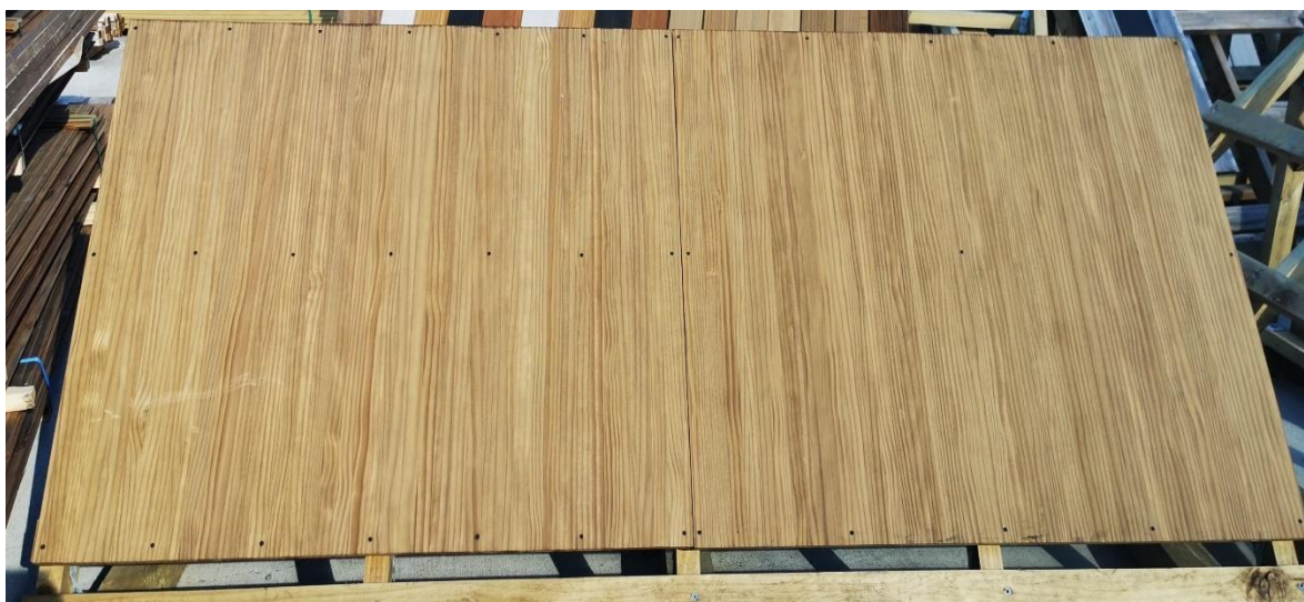
Figure 13. Mini-CLT panels weathering
