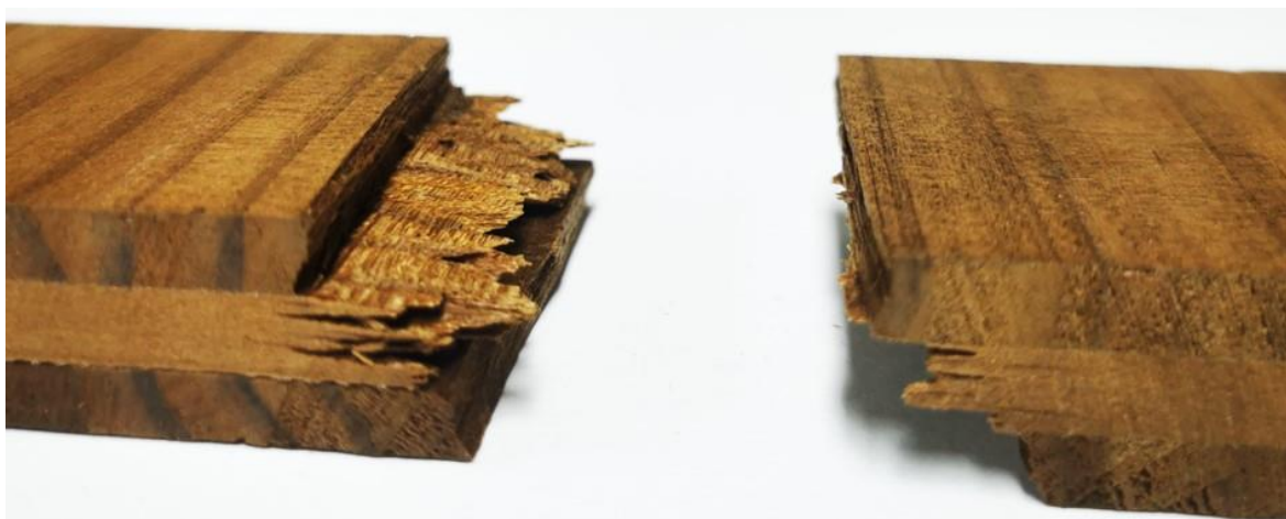
Figure 12. Mini-CLT after failure in bending
