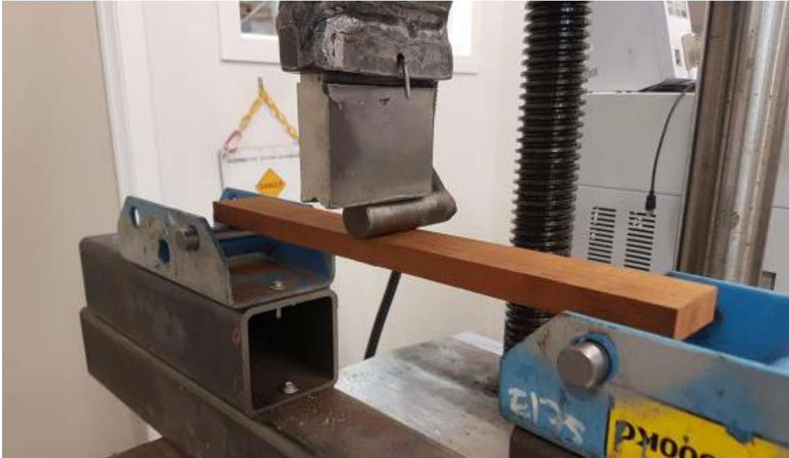
Figure 9. Glulam specimen in MOE/MOR test (Lee, 2021a)
