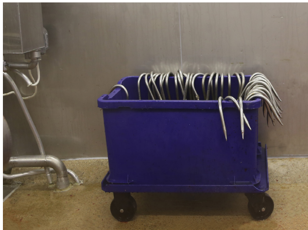
Picture 3. Meat hooks must be stored so that the hook's section touching the overhead rail does not contaminate the hook section touching the carcass.
