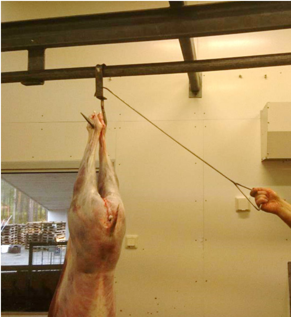
Picture 4. Carcasses are transferred from the meat hook with the help of a dedicated hook-ended tool. The hook intended for transferring carcasses is a more hygienic choice than cords for changing overhead rail lines. The hook for transferring carcasses can be thoroughly cleaned, hygiene of cords hanging at the rail junctions is most often inadequate and impossible to verify. Photograph by Sauli Laaksonen.
