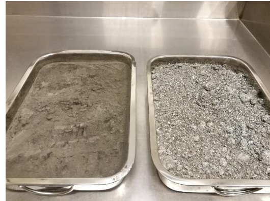
Figure 2: Grinded and unprocessed green liquor dregs.
