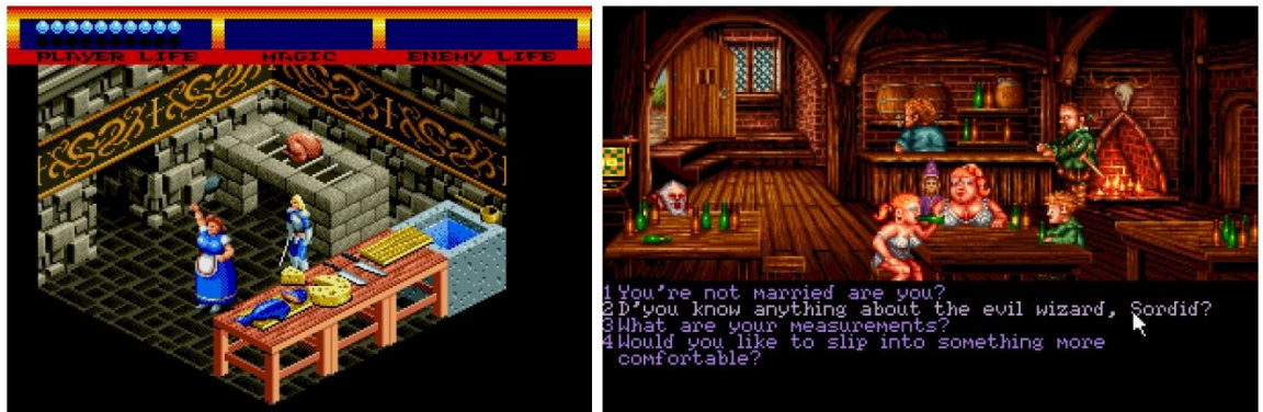
Figure 5. Parallel projection (Left) with game Light Crusader, Treasure, 1995) and Perspective projection (Right) with game Simon the Sorcerer, Adventure Soft, 1993 (Jan, Game developer's guide to graphical projections, Part 1: Introduction, 2017)
