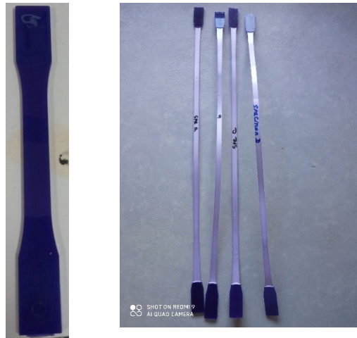
Figure 14 Tensile specimen before and after test
