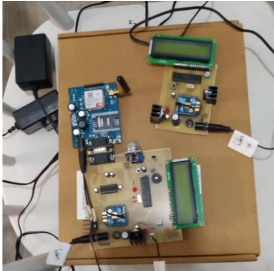
Figure 39. Gas and Fire Detection System with PCB
