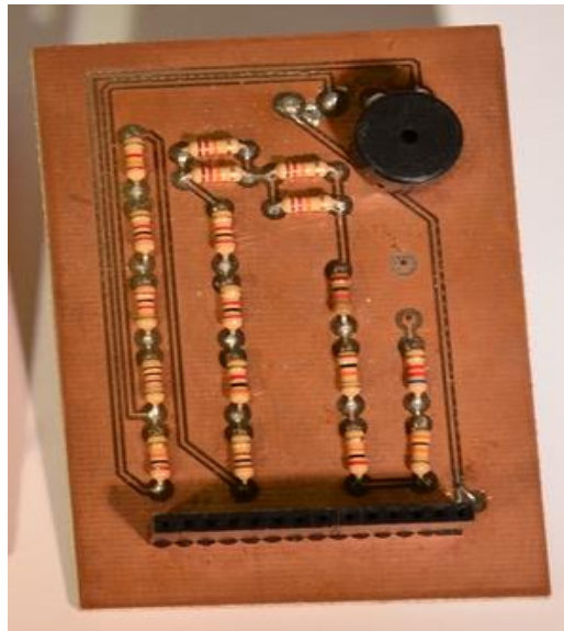
Figure 14. PCB with copper exposed [17]
