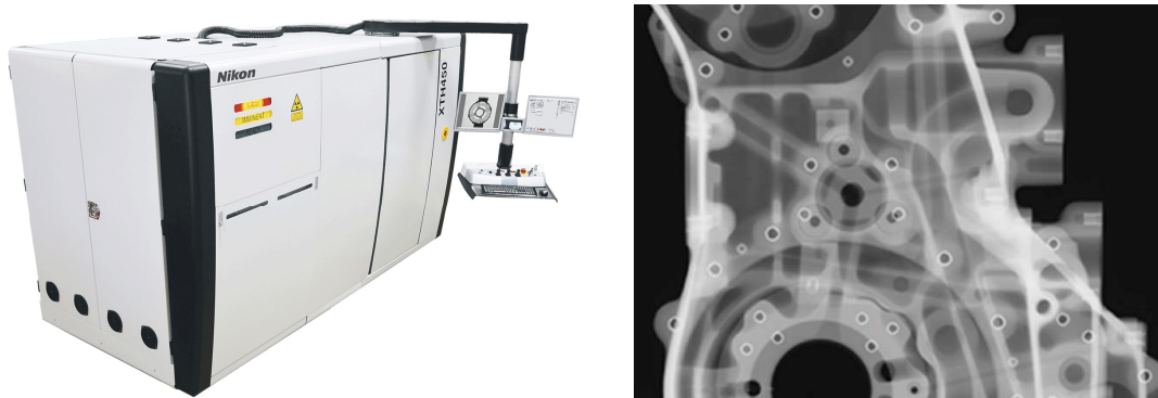
Figure 5. Nikon X-ray Inspection System and an X-ray of an engine. [9]
