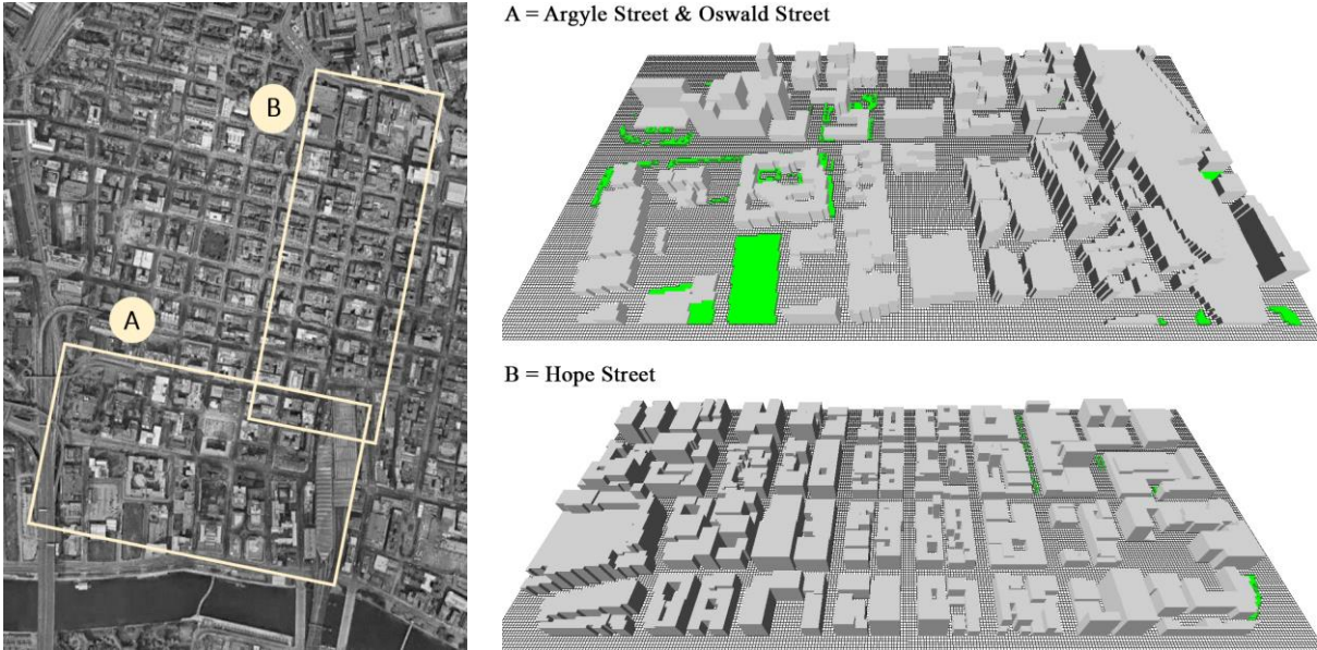
Figure 4.24 Map and models of sites A and B. Source: Google Maps, 2021; ENVI-met Version 4.4.5, 2021.
