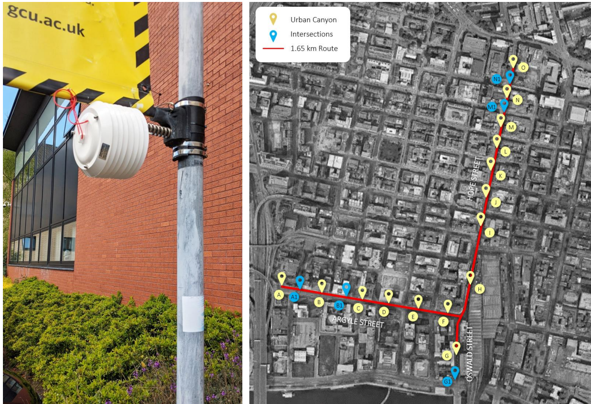
Figure 3.3 Fixed station mounted 2mts AGL (left) and routes and locations for the mobile measurement (right).
