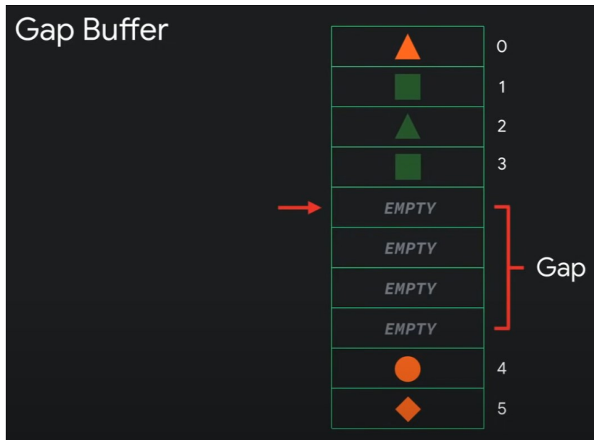
Figure 3. Gap inside the Gap Buffer is inserted in the middle of the buffer if new elements are added [13].
