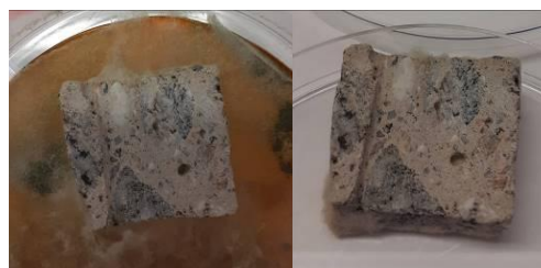
Figure 10: Example from mould growth (MKSS3 C) on the surface of test pieces at the test 2 on days 28 (left) and 56 (right). Their surface area of moulds and yeasts were monitored, which only growing on edge of the test piece.
