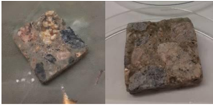
Figure 6: Example from mould growth (SSFIL A) on the top of surface of test pieces at the test 1 on days 28 (left) and 56 (right). Only moulds on the top of surface that are taken into account of processing the results.
