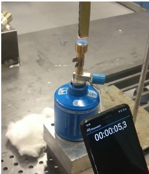
Figure 6. UL94V-0 Burning test with Bunsen burner and battery container material.
