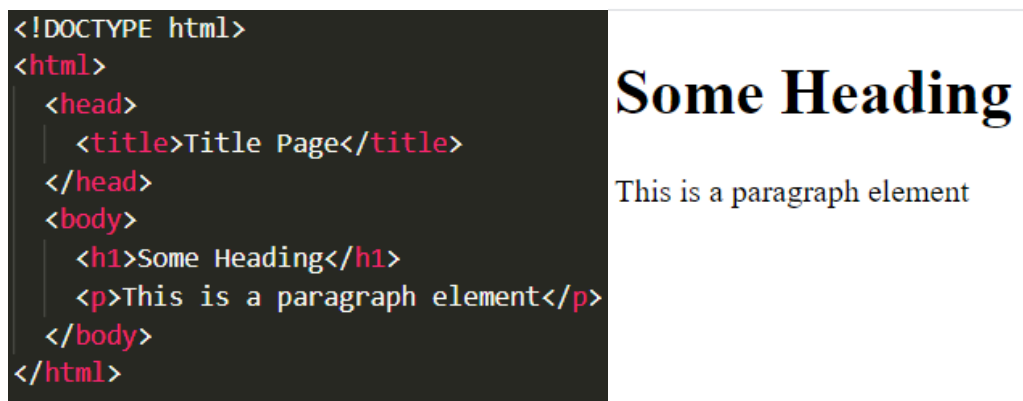
Figure 5. A simple HTML file with the title element of “Title Page”, a heading element with “Some Heading”, and a paragraph with content “This is a paragraph element”. The resulted rendered can be seen on the right image.
