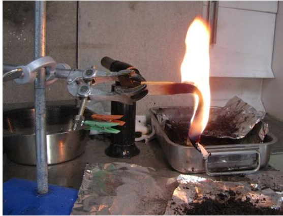
Figure 24. 100% GP50 burns without dripping. Photograph Christian Östman 2012.
