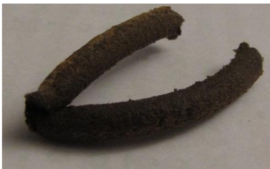
Figure 17. Burnt material, 80% GP30 + 20% Exolit AP422. Photograph Christian Östman 2012.
