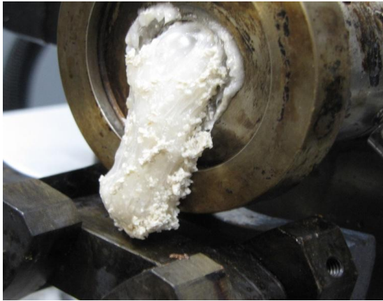
Figure 15. Extruder screw end . Photograph Christian Östman 2012.
