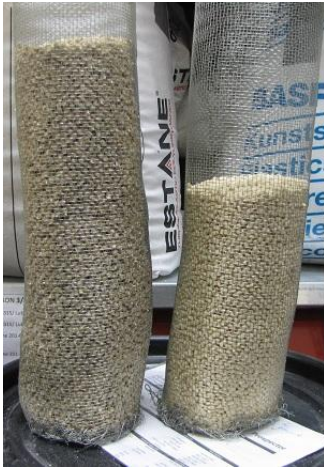
Figure 14. Extruded and non- extruded GP. Photograph Christian Östman 2012.
