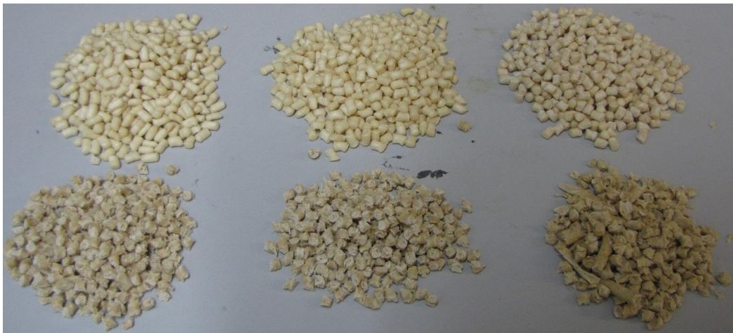
Figure 7. Upper row virgin GP, row below extruded GP. From left GP30, GP40, GP50. Photograph Christian Östman 2012.
