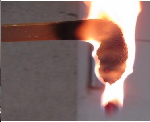
Figure 25. 80% GP30 20% Apyrum. Material dripping. Photograph Christian Östman 2012.
