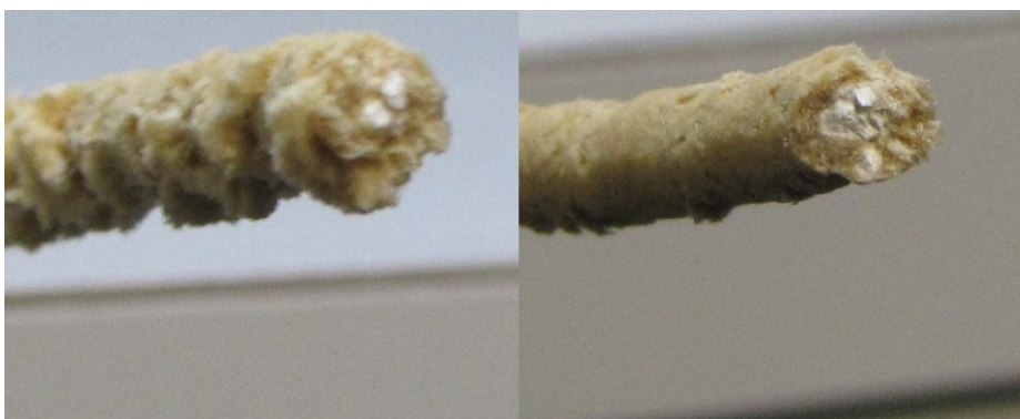
Figure 13. FR lumps and surface smoothness difference in the two extrudate strings. Photograph Christian Östman 2012.
