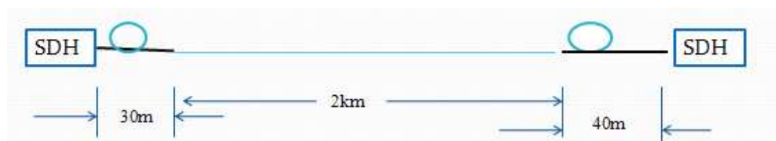
Figure 5.18. SDH Equipment with Optical Fibre Line Connection Diagram.
