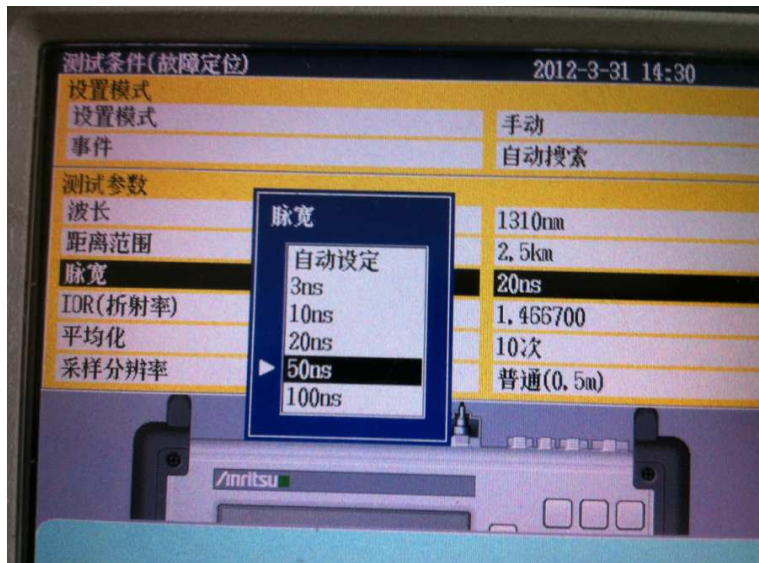
Figure 5.16. OTDR setting pulse widths with 50ns.
