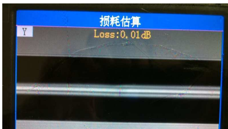
Figure 4.5. Splice loss assessment.
