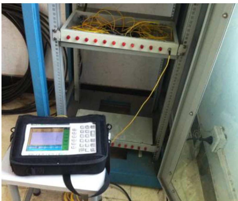
Figure 4.9. OTDR end point connecting diagram.
