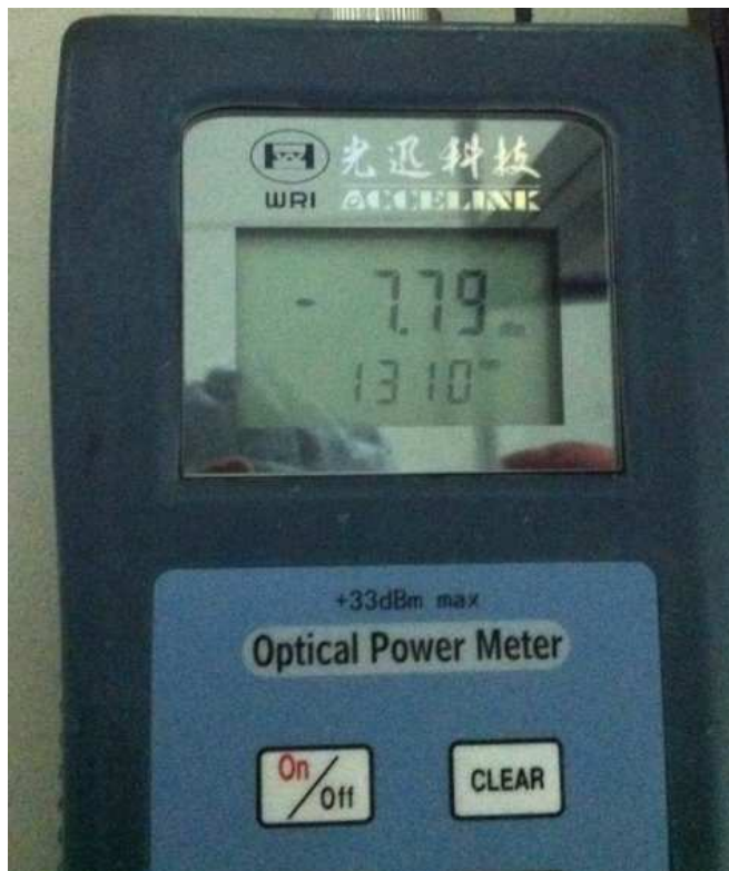
Figure 5.8. The Optical Power Meter Value.
