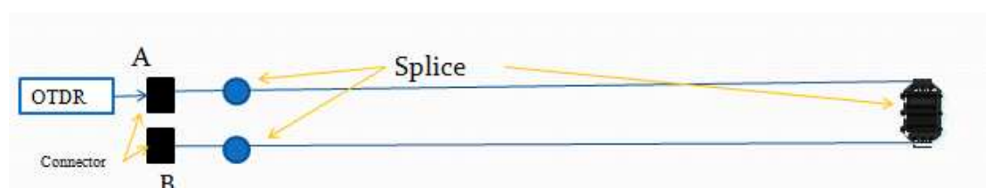
Figure 4.1. Optical fibre cable distribution in real test.
