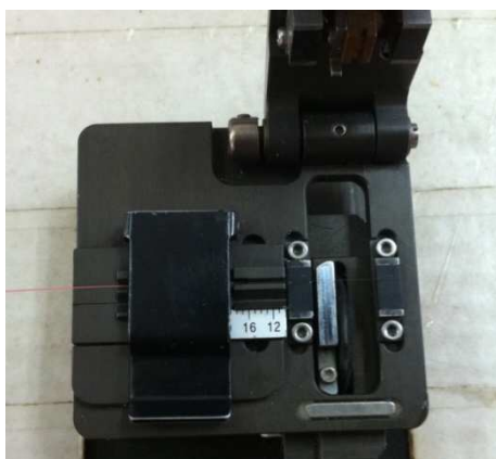
Figure 4.3. The fibre end face cutting diagram.
