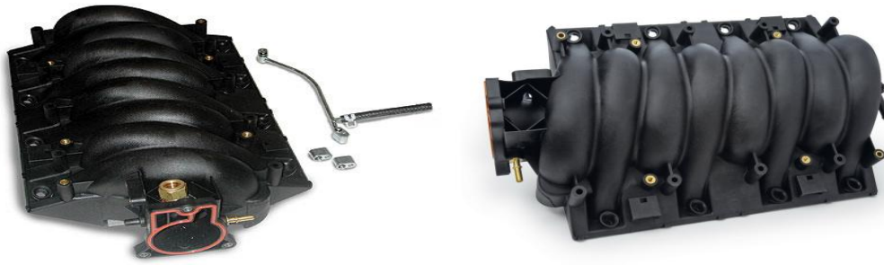
Figure 7: A carbon fiber reinforced PA manifold, [10]
