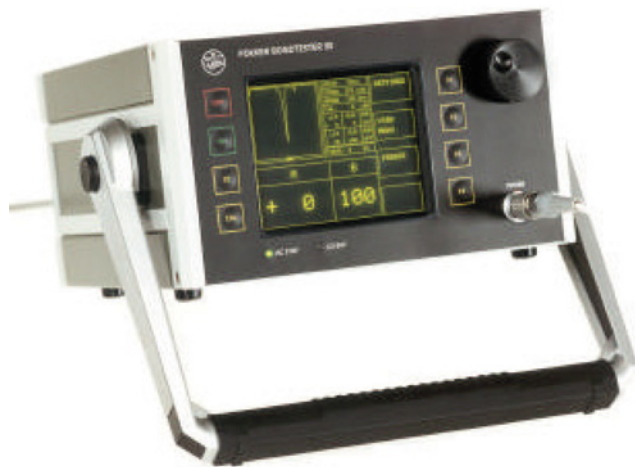
Figure 9. Fokker Bondtester Model 90 is a bond tester that employs membrane resonance method to test the bonds. /10/
