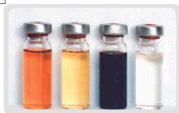
Picture from left: Mineral oil (ASTM 565), mineral oil (JECFA), unpurified Polydecene and Hydrogenated Polydecene (Alphaflow®)
