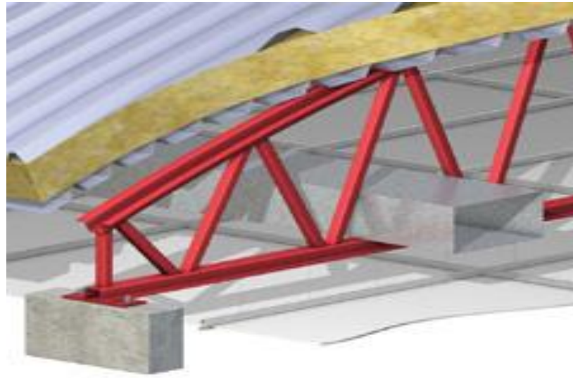
Figure 5. lattice roof beam
