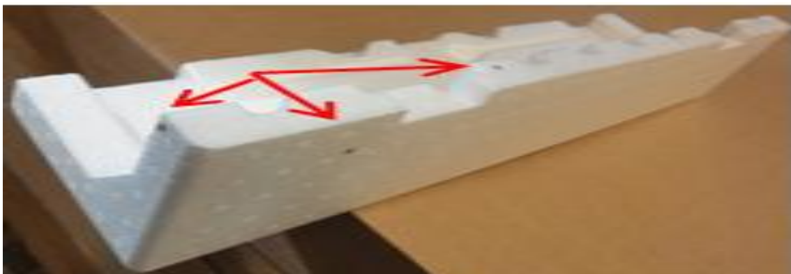
FIGURE 6. Visual defect in cushion
