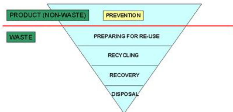
FIGURE 4. Waste management hierarchy (EU Waste Framework Directive 2008/98/EC)
