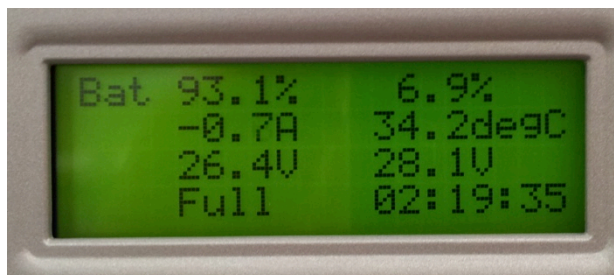
PICTURE 16. Absorption phase of battery charging
