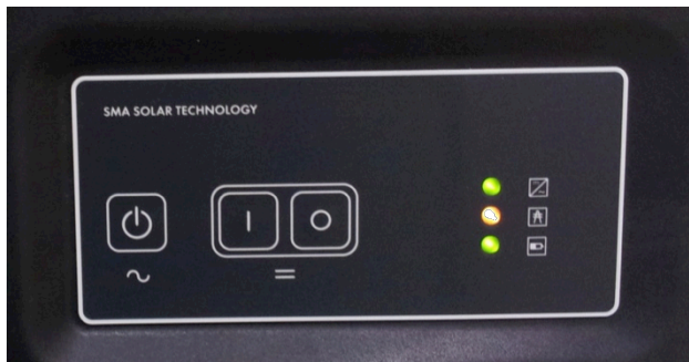
PICTURE 18. Synchronisation of feed grid or generator
