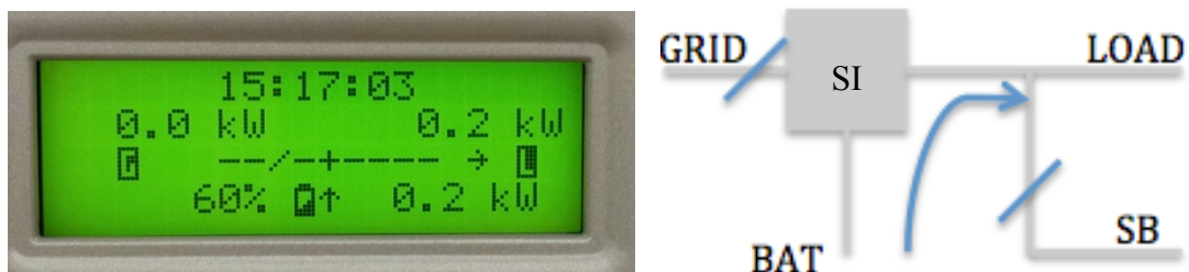
PICTURE 19. Feeding stand-alone grid from the batteries
