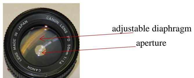
Figure 10 showing adjustable diaphragm (Pokharel, 2013)
