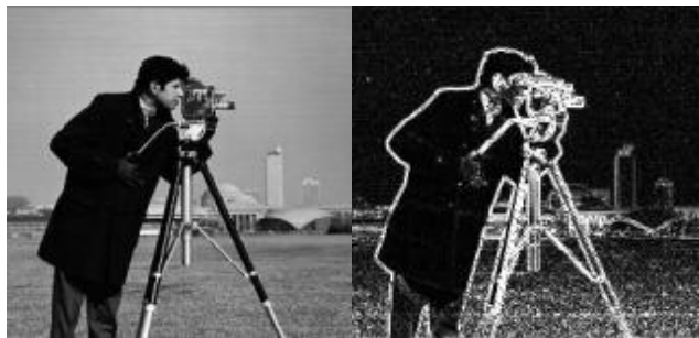
Figure 20 Images before and after edge formation (National Instruments)
