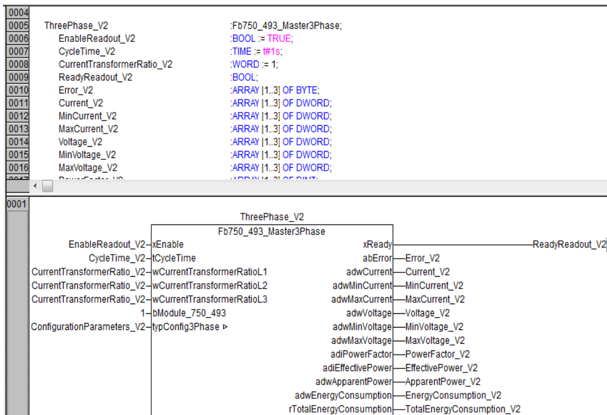
Figur 11. Programmet "Measuring3Phase" med blocket "Fb750_493_Master3Phase".
