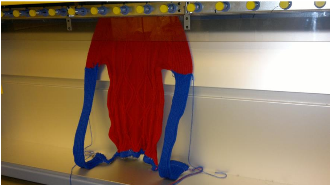
Picture 1. 3D knitwear prototype production in Stoll machine.
