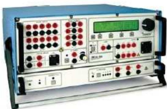
Figur 3. Megger Freja 306, Relä test system /4/
