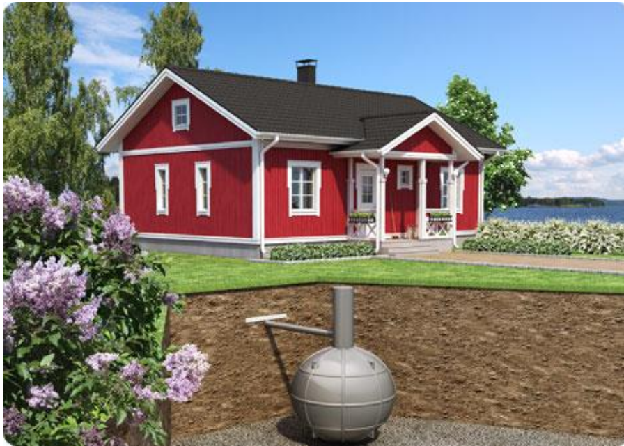
FIGURE 3 Closed tanks store wastewater from households ( http://www.ecolator.fi/tuotteet/umpisailio )
