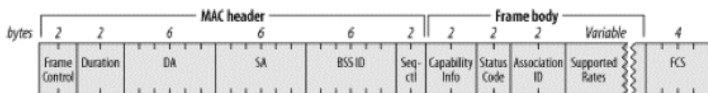
Figure 19. Reassociation response frame header
