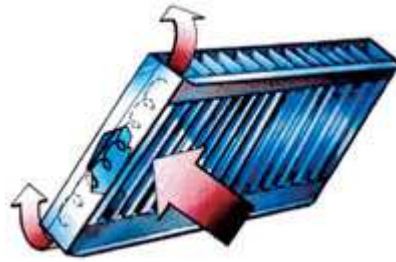
Figure 11 Structure of a multicyclone filter /8/
