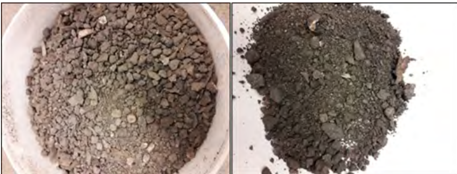
FIGURE 1. Incineration bottom ash (IBA) sample delivered to FiberLaboratory; IBA is fractionated with 16 mm hole screen (Photo Irina Turku).
