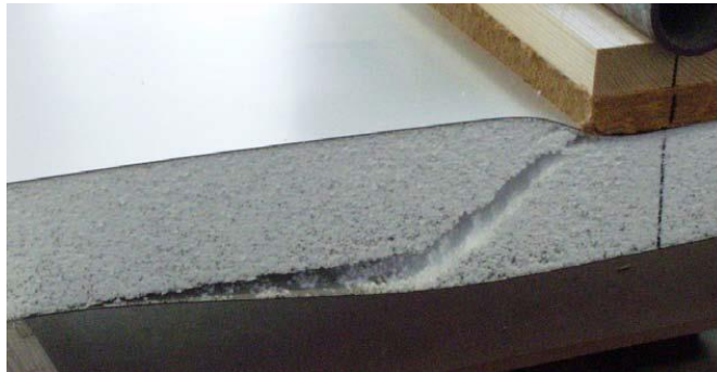
Figure 4a Wrinkling of the compressed face (EASIE 2011)
