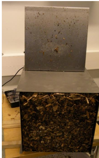
Figure 18. Sprayed silicone oil on steel
