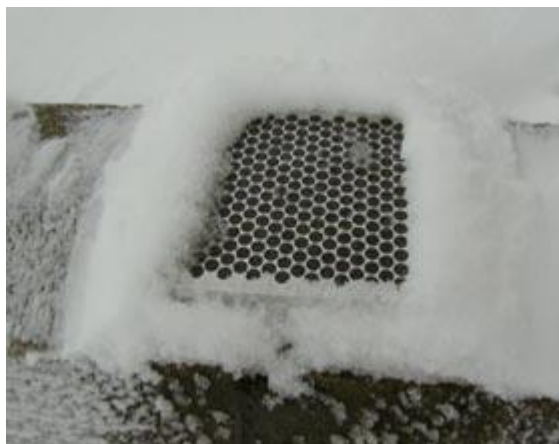
Figure 1. Icewick Anti-icing Grate prototype melting snow (IDI 2007)
