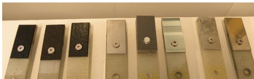
Figure 22. Results sample after the CAT tests. From left to right, TS-SLIPS, rough FS-PE, smooth FS-PE, steel and silicone oil, Quicksilver PE, PTFE tape, steel, steel and anti-freeze.
