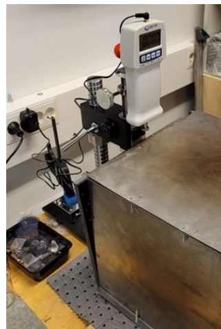
Figure 6. Set up for shear tests at room temperature with force gauge
