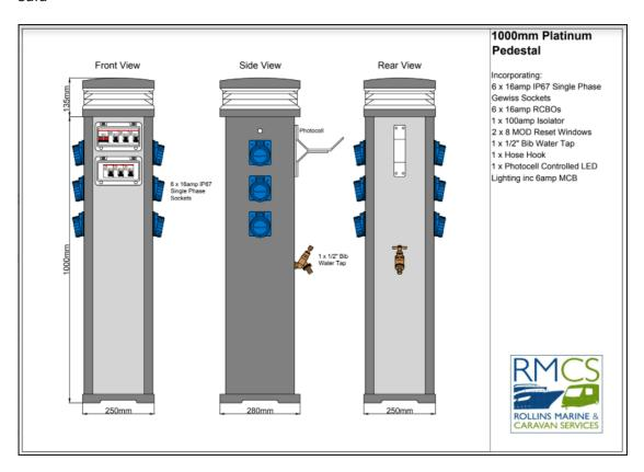
Figure 11. Specifications of the service stands installed in Lennusadam piers.
