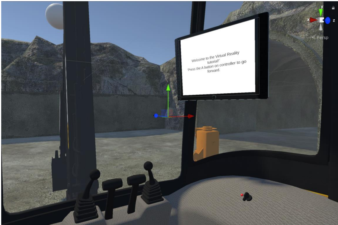
Figure 14. A monitor displays instructions to the player inside the excavator cabin.
