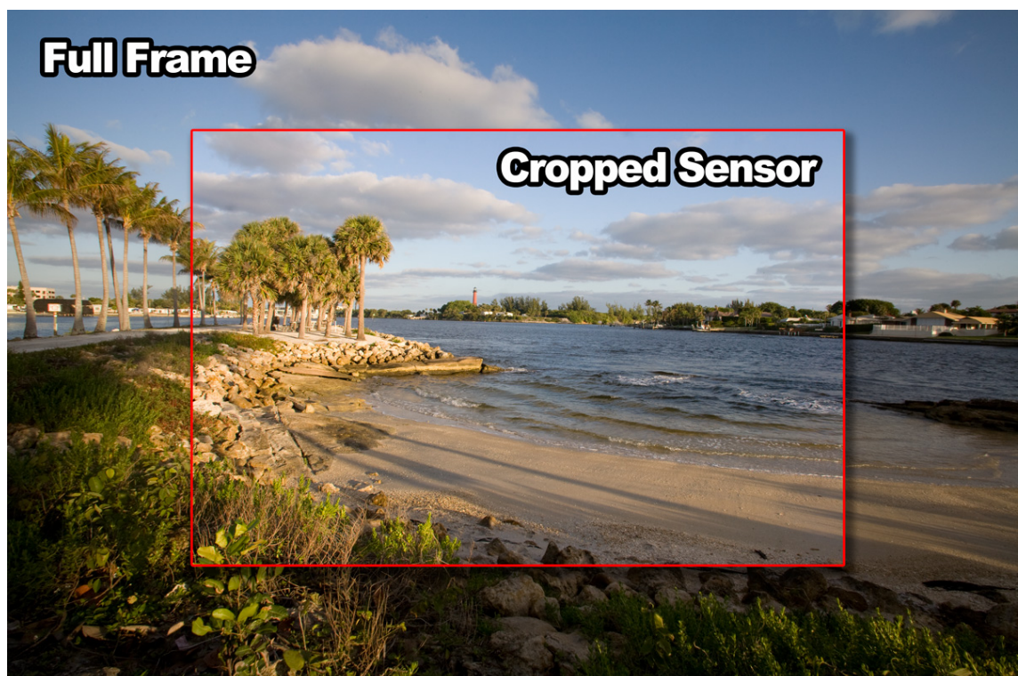
PICTURE 1. The APS-C sensor is often called a crop sensor because in a way it crops out a part of the scene compared to a full frame sensor (Captankimo 2013)
