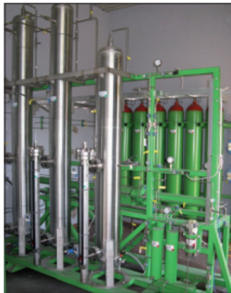
FIGURE 29. The patented Metener biogas upgrading technology in Kalmari farm (Motiva Ltd, 2012)
