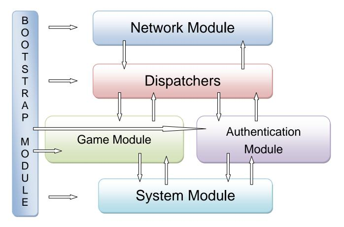
Figure 8. Tiers of the server software architecture
