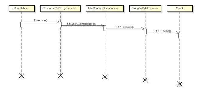
Figure 10. Sequence diagram for network module response processing
