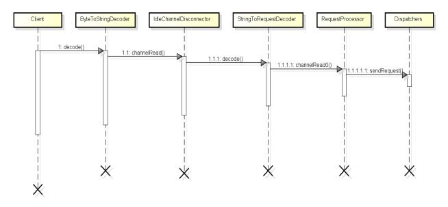
which constructs a Java request object out of the given character data. RequestProcessor decides to which dispatcher the particular request should be sent to.
