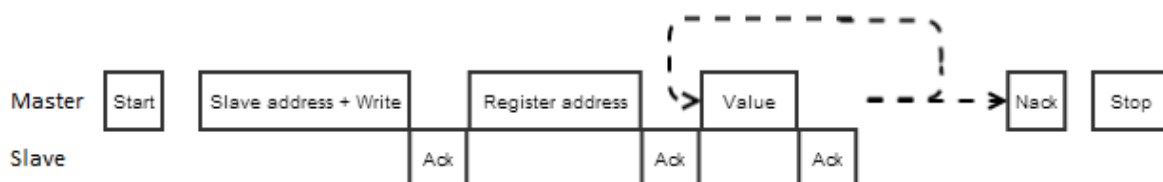
FIGURE 3 I2C_dataWrite logic (Arponen 2014.04.04)
