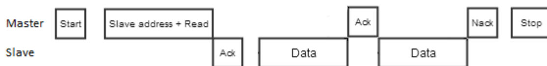
FIGURE 21 Barometer data fetch (Arponen 2014.04.04)
