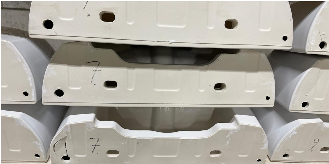
Figure 33: Cracks from drilled feed hole
