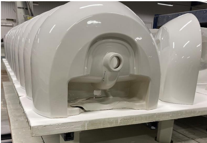
Figure 22: Crack after firing
