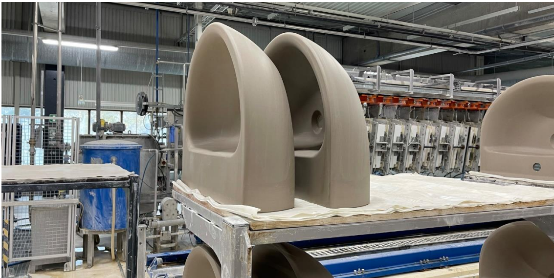
Figure 20: Drying cart and washbasins
