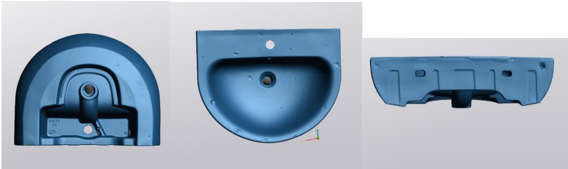
Figure 42: M5 scanned with Creaform Handyscan BLACK 3D
