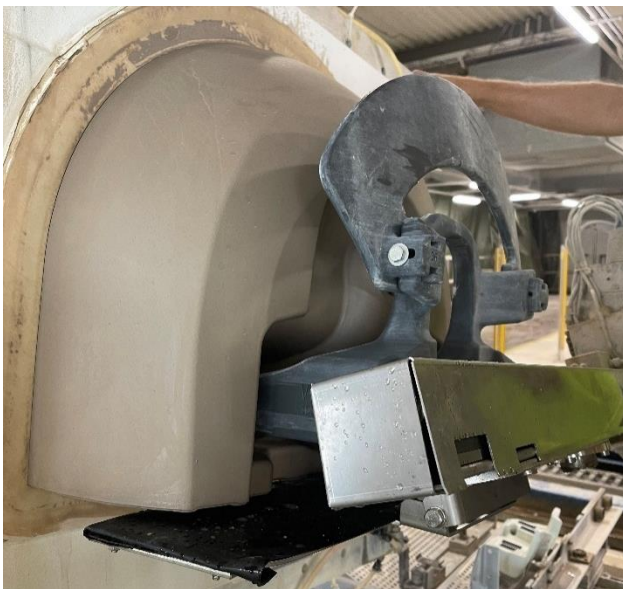
Figure 31: Resetting de-moulding angle
