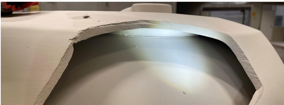
Figure 18: Crack along the hollow and solid cast edge, jagged
