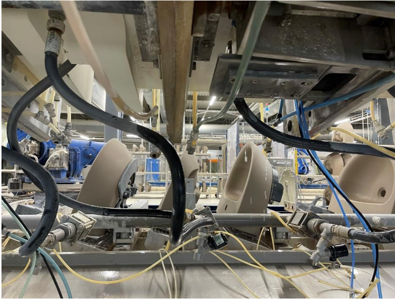
Figure 9: External mould piping
