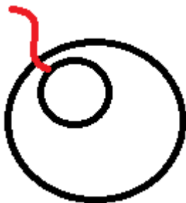
Figure 49: Crack direction(red) depending on the drilling offset from feed
