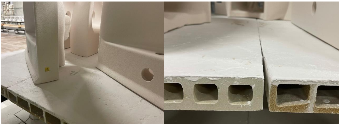
Figure 36: Kiln cart in bad condition
