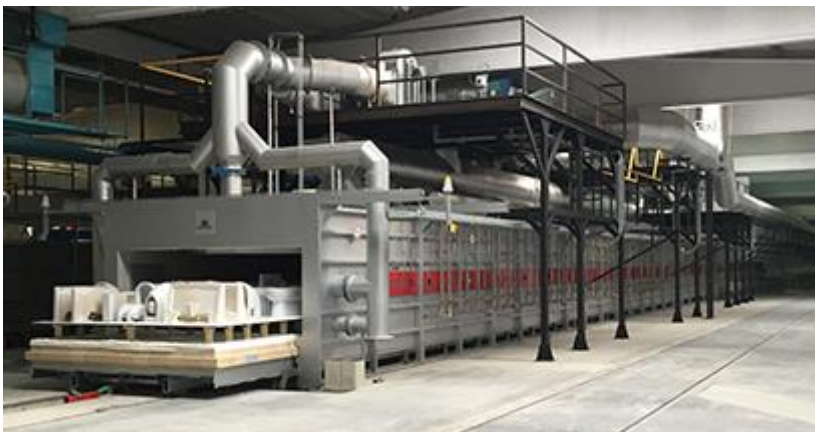
Figure 15: Riedhammer tunnel kiln (Source: Ceramic World Web)
