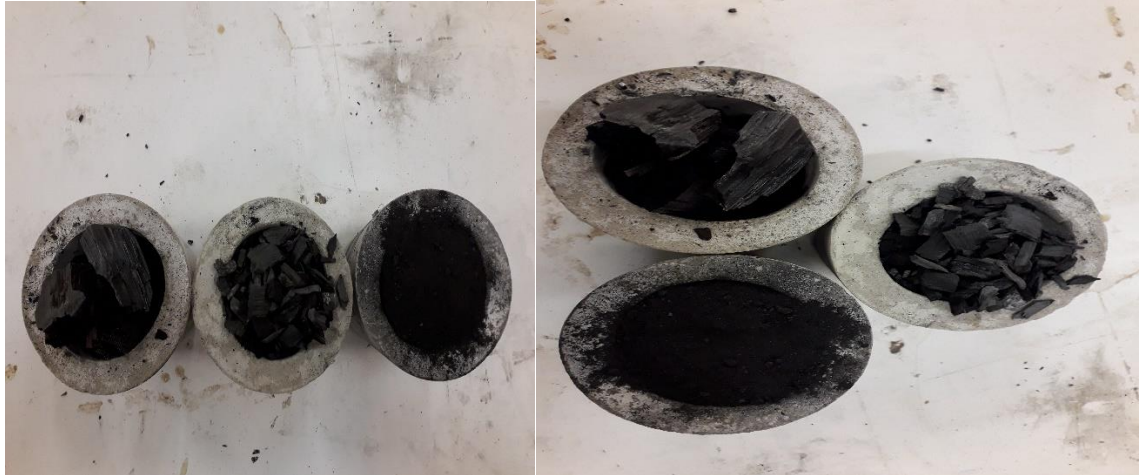
Figure 5 On the left is the SoilCare biochar blocks before and after grinded. On the right is the Carbo Culture pine wood chips biochar before and after grounded (Tuominen 2021).
