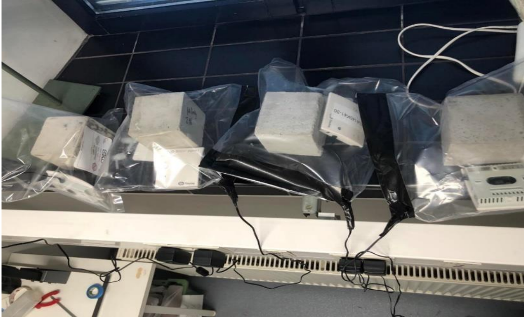
Figure 11 Experimental setup that was used for the identification of the carbon sequestration property
