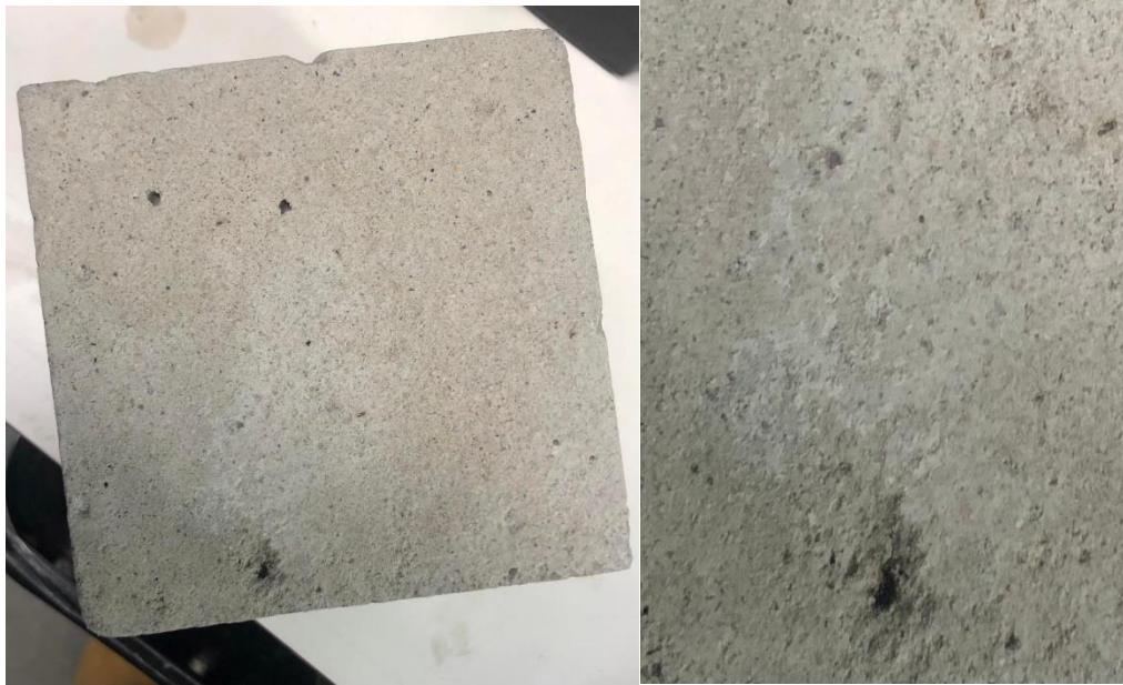
Figure 13 Agglomeration of biochar in the concrete (Tuominen 2021)
