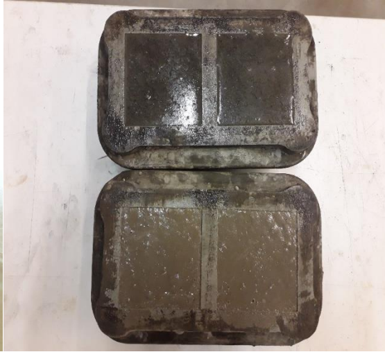
Figure 7 Specimen molding - At the top is 10 wt% biochar mixture and at the bottom is a plain concrete (Tuominen 2021).
