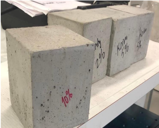
Figure 8 Concrete cubes with different percentage of biochar (Tuominen 2021)
