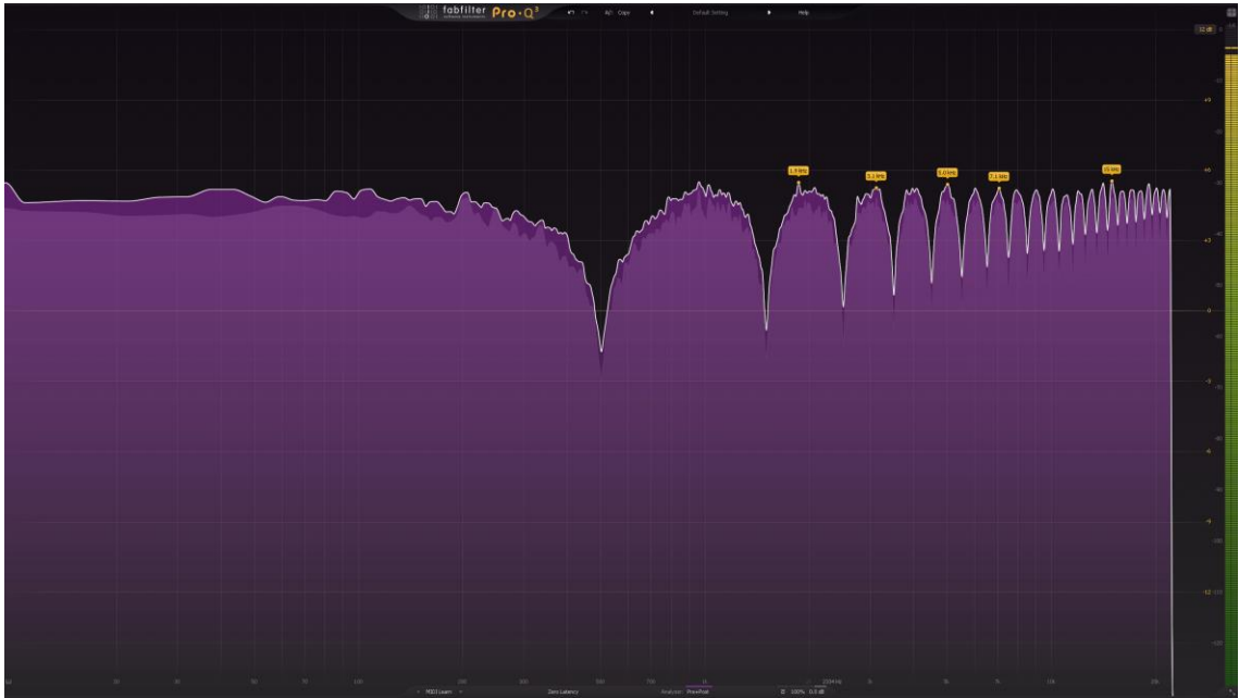
PICTURE 6. Comb filtering as a result of two channels of pink noise when one of them is delayed by 1 millisecond. The analyser has been set to 3 dB per octave tilt (Seppänen 2022)
