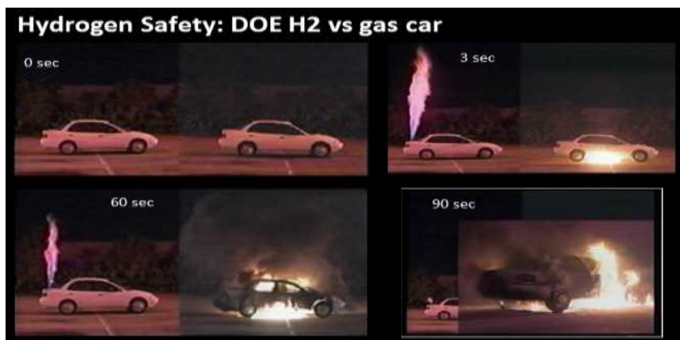
Figure 12. Hydrogen safety, the explosion of a hydrogen car (left picture) vs gas car (right picture), (Leachman 2017).
