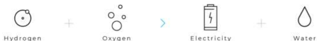
Figure 10. Fuel cell that uses hydrogen to generate electricity. How it works. (Nikola Motor 2022)
