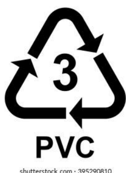
PICTURE 13: Polyvinyl Chloride (PVC) resin identification code (Shutterstock, N.d. Used with permission.)
