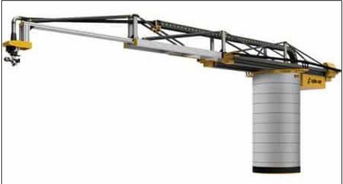
Figure 6. crane system for 3DCP by Apis Cor (Aniwa Pte. Ltd. 2022)
