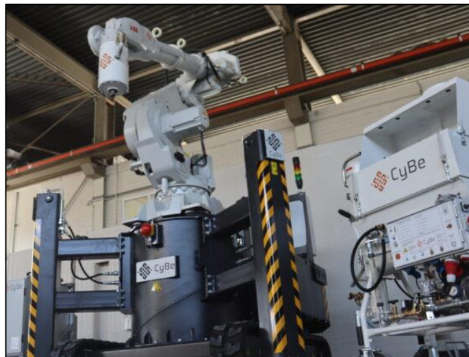
Figure 5. moveable robotic system for 3DCP (CyBe Construction 2022)
