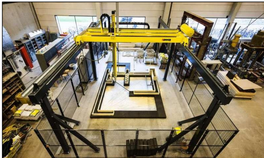
Figure 3. Gantry system for 3DCP at TU Eindhoven (3dprinter.com 2022)
