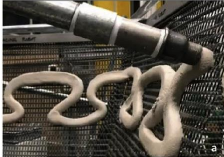
Figure 13. Extruding concrete onto a previously placed carbon mesh grid (Mechtcherine et al. 2020)
