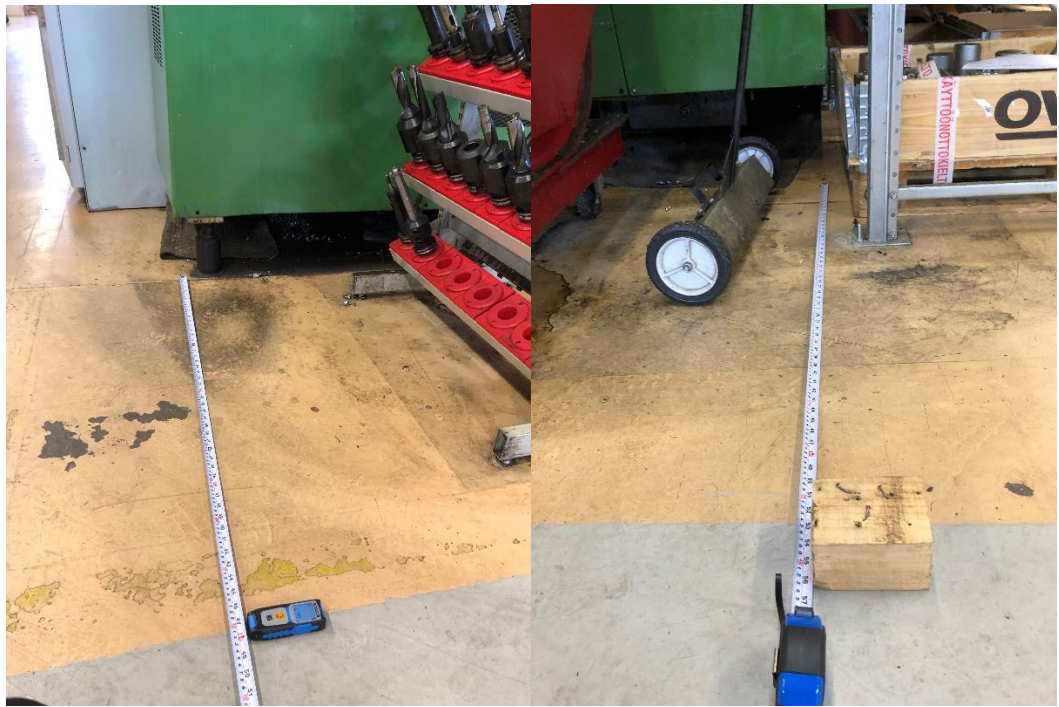
Figure 15. Placing the laser (Left) and placing the reflector (Right). (Huang, 2022)
